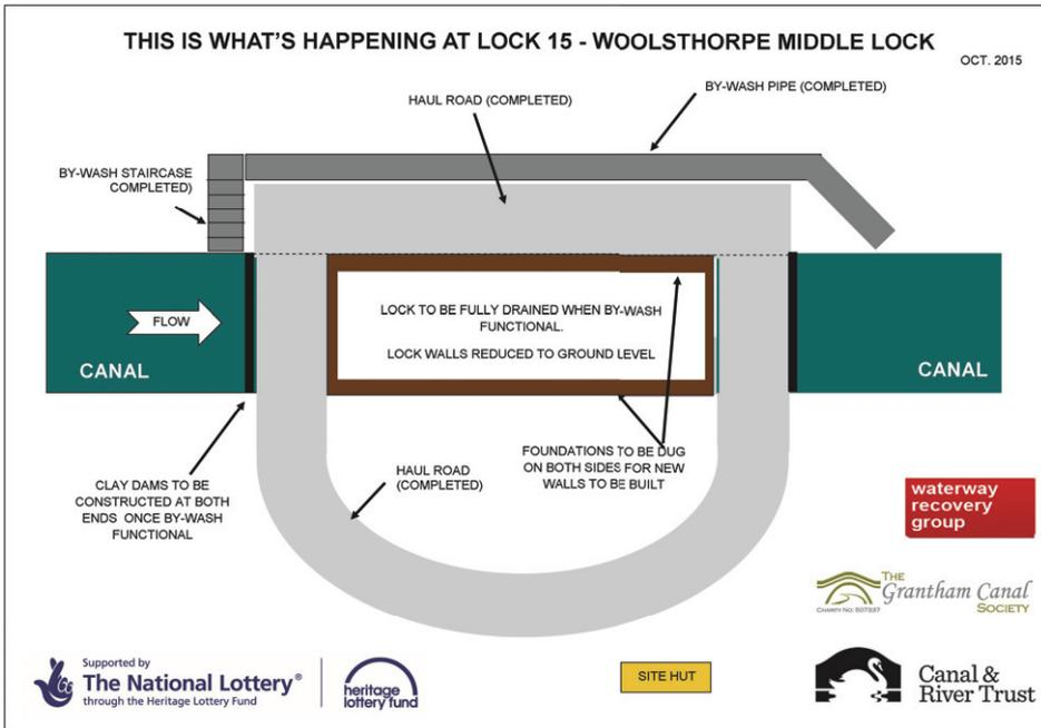
The current 'state of play' is that before the by-wash can be used the concrete has to cure. It will then have the final brickwork completed before the canal can be dammed.
