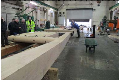
Two photos taken by John Clark of lock gates under construction in the CRT factory
